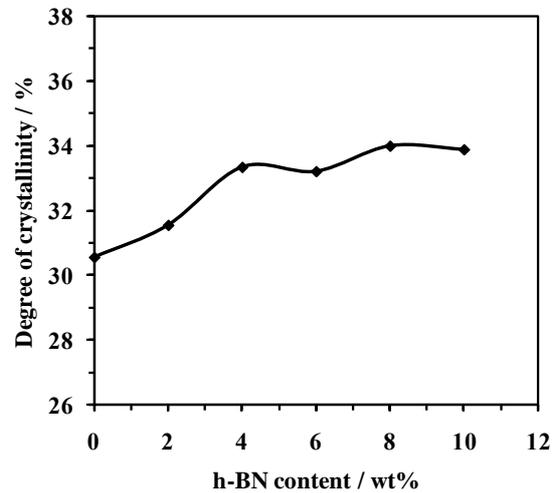
**Figure 7** Degree of crystalline of PEEK and h-BN/PEEK coatings
