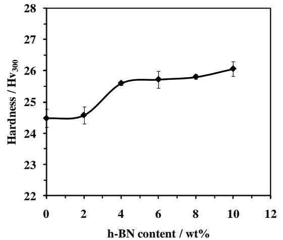
**Figure 6** Hardness values of PEEK and h-BN/PEEK coatings
