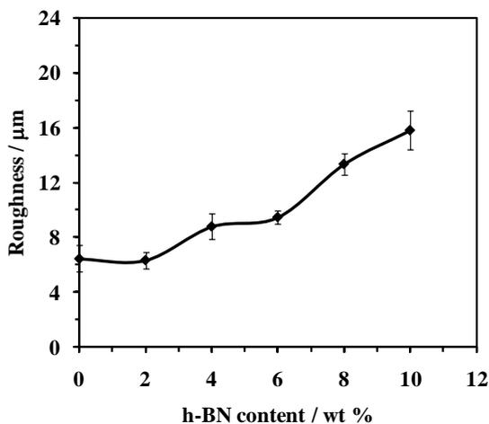
**Figure 5** Surface roughness measurements of PEEK and h-BN/PEEK coatings
