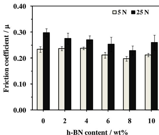
**Figure 10** Average friction coefficients of PEEK and h-BN/PEEK coatings
