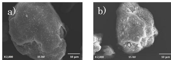
**Figure 2** SEM images of a) 2 wt% h-BN/PEEK; and b) 10 wt% h-BN/PEEK
