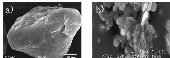
Figure 1 SEM images of a) PEEK; and
