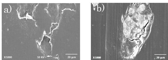
**Figure 9** SEM images of the worn surfaces of 10 wt% h-BN/PEEK coating under a load of a) 5N and b) 25N
