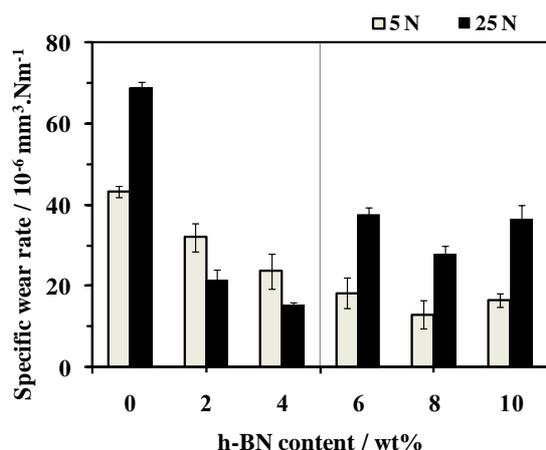
**Figure 8** Specific wear rates of PEEK and h-BN/PEEK coatings
