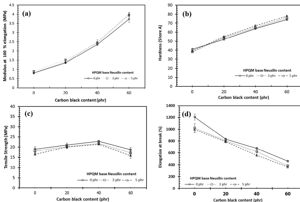
**Figure 1** Mechanical properties of NR rubber compound filled carbon black and HPQM base Neusilin (a) tensile modulus (b) hardness (c) tensile strength and (d) elongation at break
