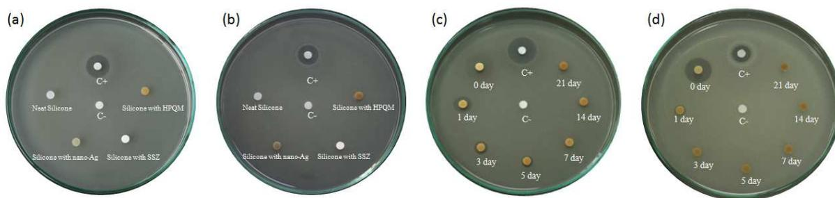
**Figure 1.** Effects of antibacterial agent type and UV aging on clear zone by Halo test. (a) and (b) silicone with various antibacterial agents at 21 day UV and 15 phr loading for *E. coli* and *S. aureus*, respectively, (c) and (d) silicone with HPQM at 15 phr loading for various UV aging times for *E. coli*, and *S. aureus*, respectively
