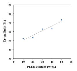
**Figure 4.** The effect of PEEK content on crytallinity of PEEK/PTFE composite coatings.
