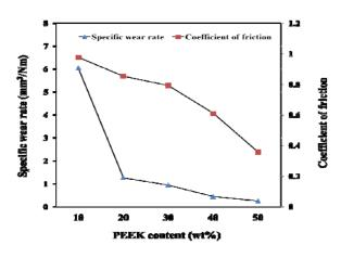
**Figure 5**. Variations in coefficient of friction and specific wear rate as a function of PEEK content (test condition: load 1N, sliding speed 0.1 m/s).
