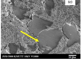
**Figure 6**. Worn surfaces of the PEEK/PTFE composite coatings (a) 30 wt%, (b) 40 wt% and (c) 50 wt% of PEEK (test condition: load 1N, sliding speed 0.1 m/s).
