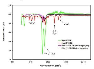
**Figure 2.** ATR-FTIR spectra for neat PTFE, neat PEEK and the PTFE composite coating with 30 wt% PEEK contents before and after spraying.
