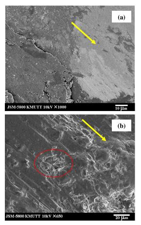
**Figure 7**. Worn surfaces of the PEEK/PTFE composite coatings with 50 wt% of PEEK after testing with different load (a) 1 N and (b) 3 N.
