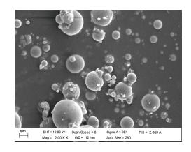
Figure 1 SEM micrograph of FA particles used in the present study
